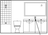
ONE RECEPTACLE CAN MEET THE — REQUIREMENT IF 3' OF THE OUTSIDE EDGE OF EACH BASIN
