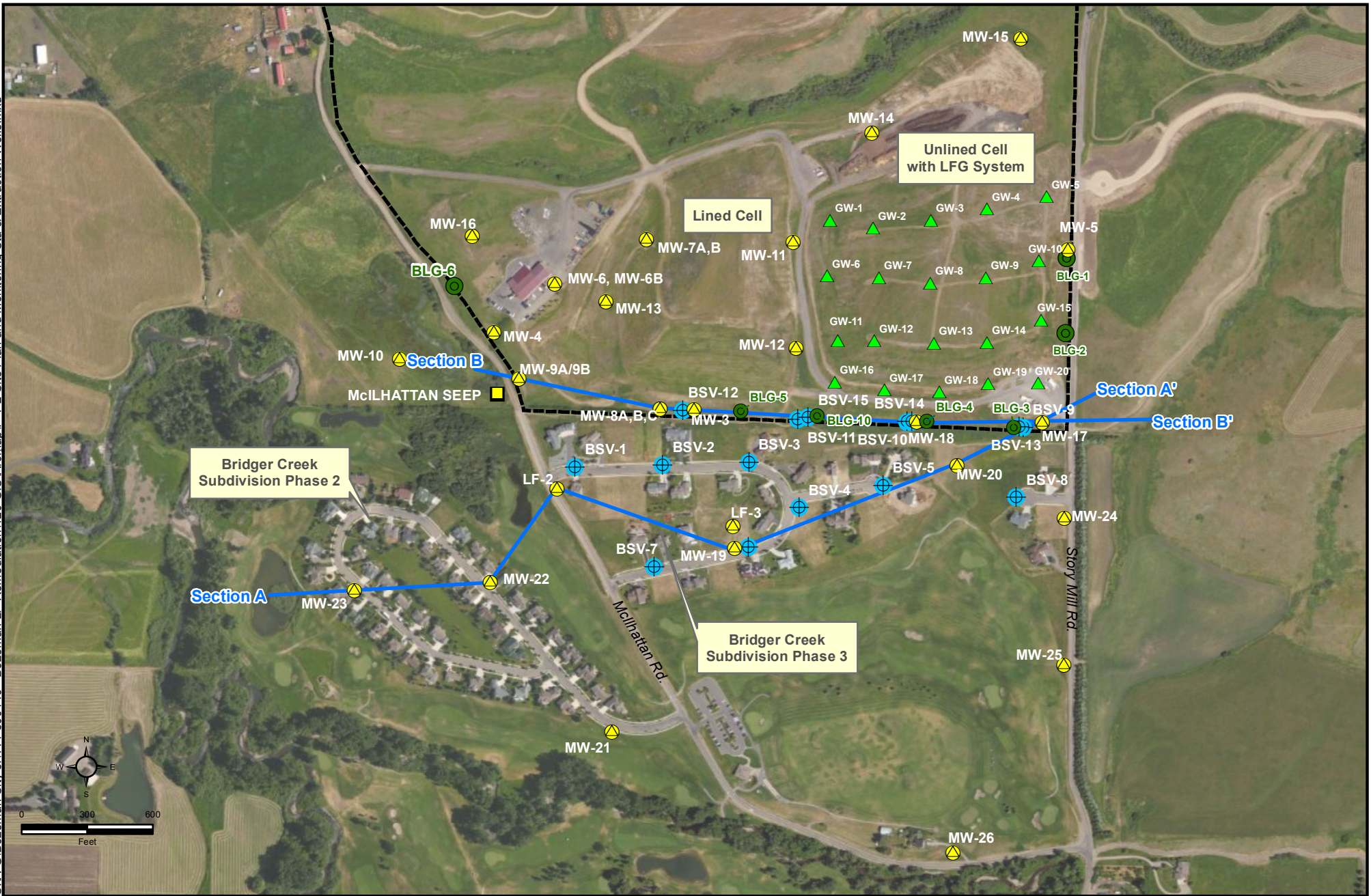
Site Plan with Monitoring Stations and Extraction Wells Bozeman Landfill Bozeman, Montana FIGURE 1-2
