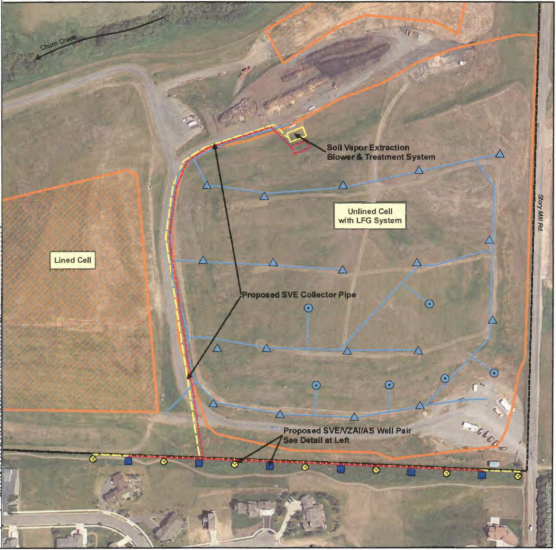
Conceptual SVE, Vadose Zone Air Injection/Air Sparging & Additional Landfill Gas Extraction Well Revised Corrective Measures Assessment City of Bozeman Landfill Bozeman, Montana
