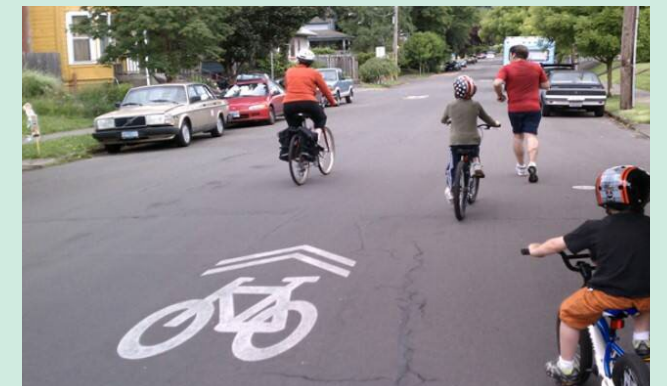
Figure 4.9 Sharrow pavement markings
