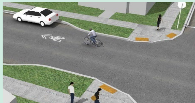
Figure 4.18 Curb bulb outs
