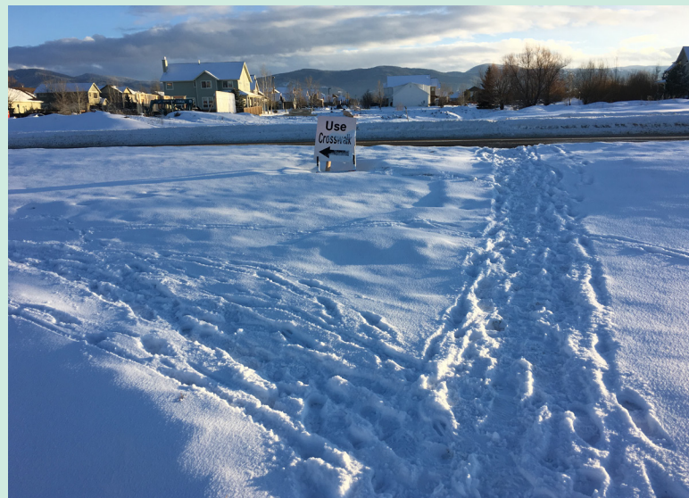
Figure 4.26 The Gallagator trail at Graf Street where trail has been cut for road extension. Snow tracks after a few hours of use show that the sign routing users to a crosswalk 160 feet away is not effective.
