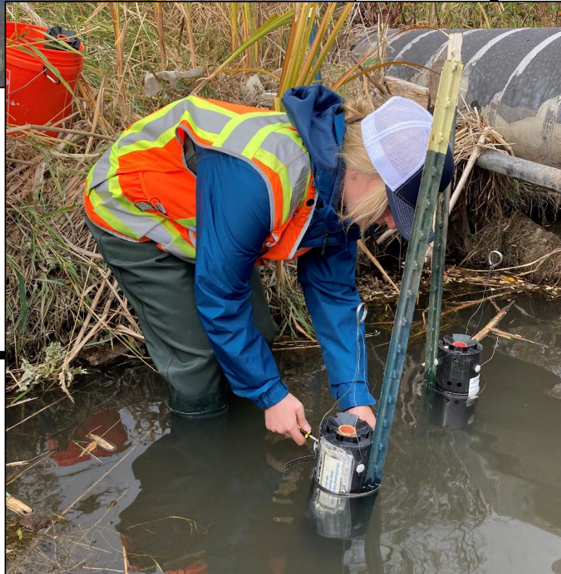
Graphic 8.0.2: Installing in-stream sampling equipment
