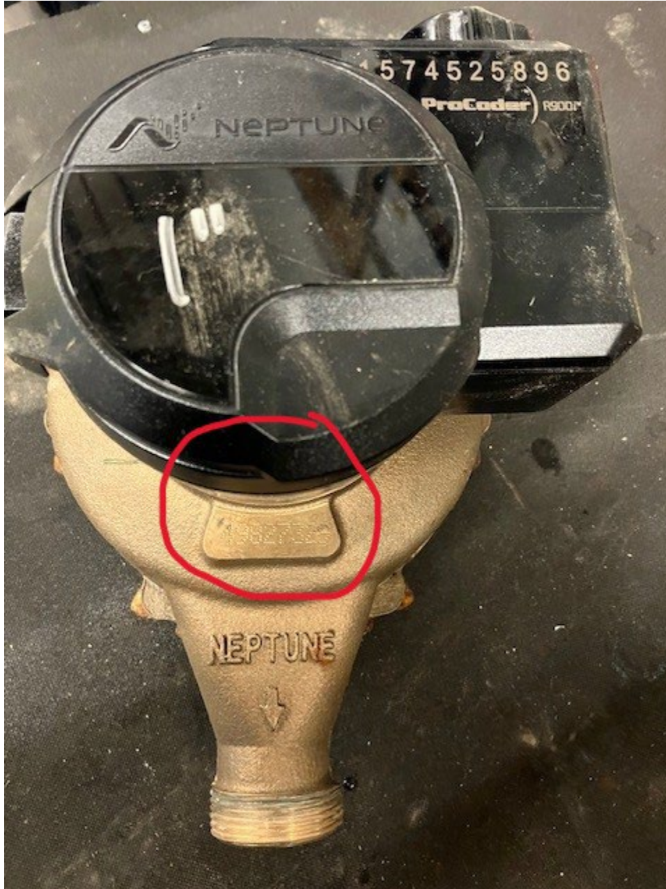
Positive displacement meters, sizes 1" * & 5/8" (3/4"), with meter serial number on brass body.
