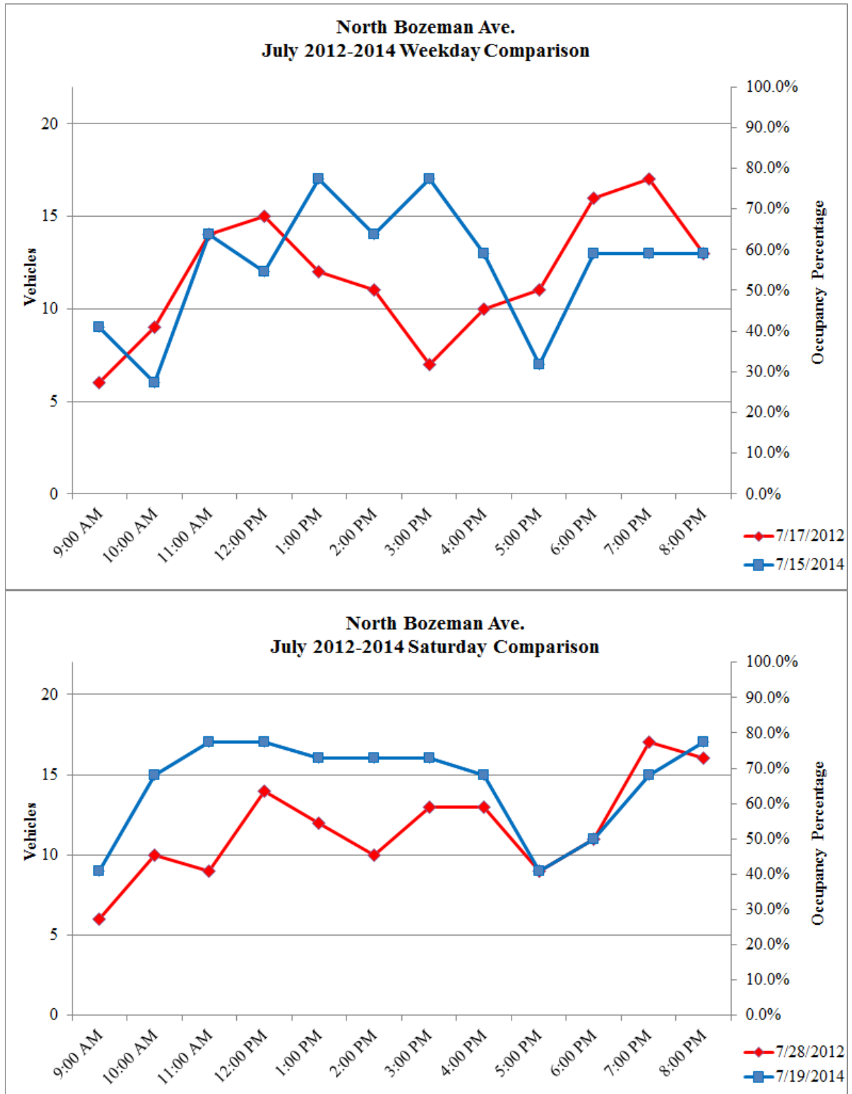
Figure 2-19: Comparison of North Bozeman Ave. occupancy rates for weekdays and weekends, July 2012 and 2014
