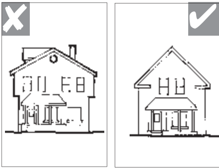
The drawing on the left shows a structure which does not relate well in mass and scale to the adjacent structure.
