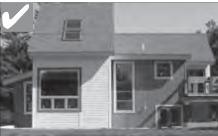
On larger structures, subdivide larger masses into smaller “modules” that are similar in size to single household residences seen historically.
