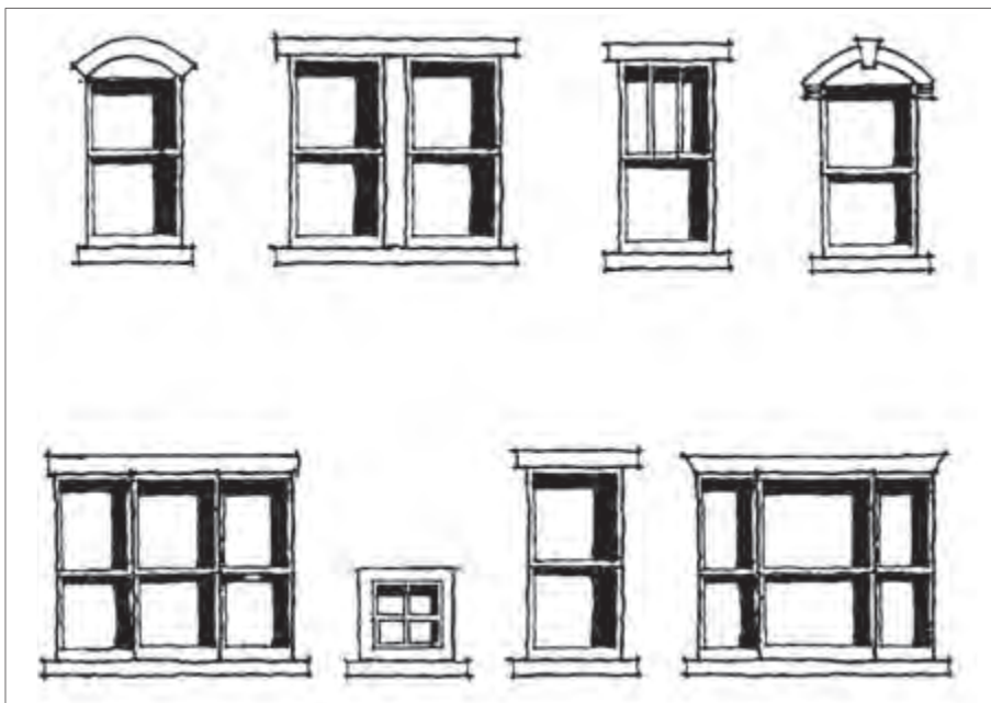
Typical primary window types seen on historic structures.
